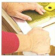
Use the edge of the 1x6 for bending along the score line. Push downward with a crisp snapping motion.
