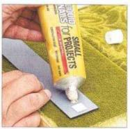
Keep the dab of adhesive small and away from edges. It dries quickly, so place the strip immediately.
