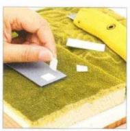
For the horizontal strips, apply a second layer of tape to compensate for the thickness of the mirror's fasteners.
