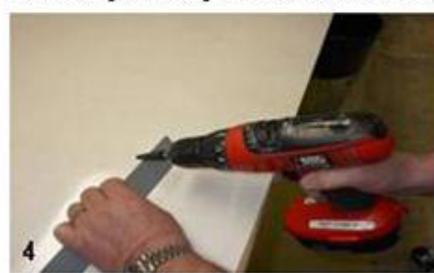
With Drill Machine and Tapered Rotary Rasp, Start a Gouge in the Mirr.Edge Strip to Accommodate the Clips
